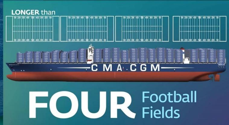
The massive Benjamin Franklin was **turned in 56 hours** of operations, averaging 29.1 lifts per crane, per hour, averaging total **200 container moves against the vessel each hour**, for a total of 11,200 lifts. The APM Terminal in Los Angeles worked as many **as nine ship-to-shore cranes simultaneously** against the Benjamin Franklin during its three and one-half day call.
