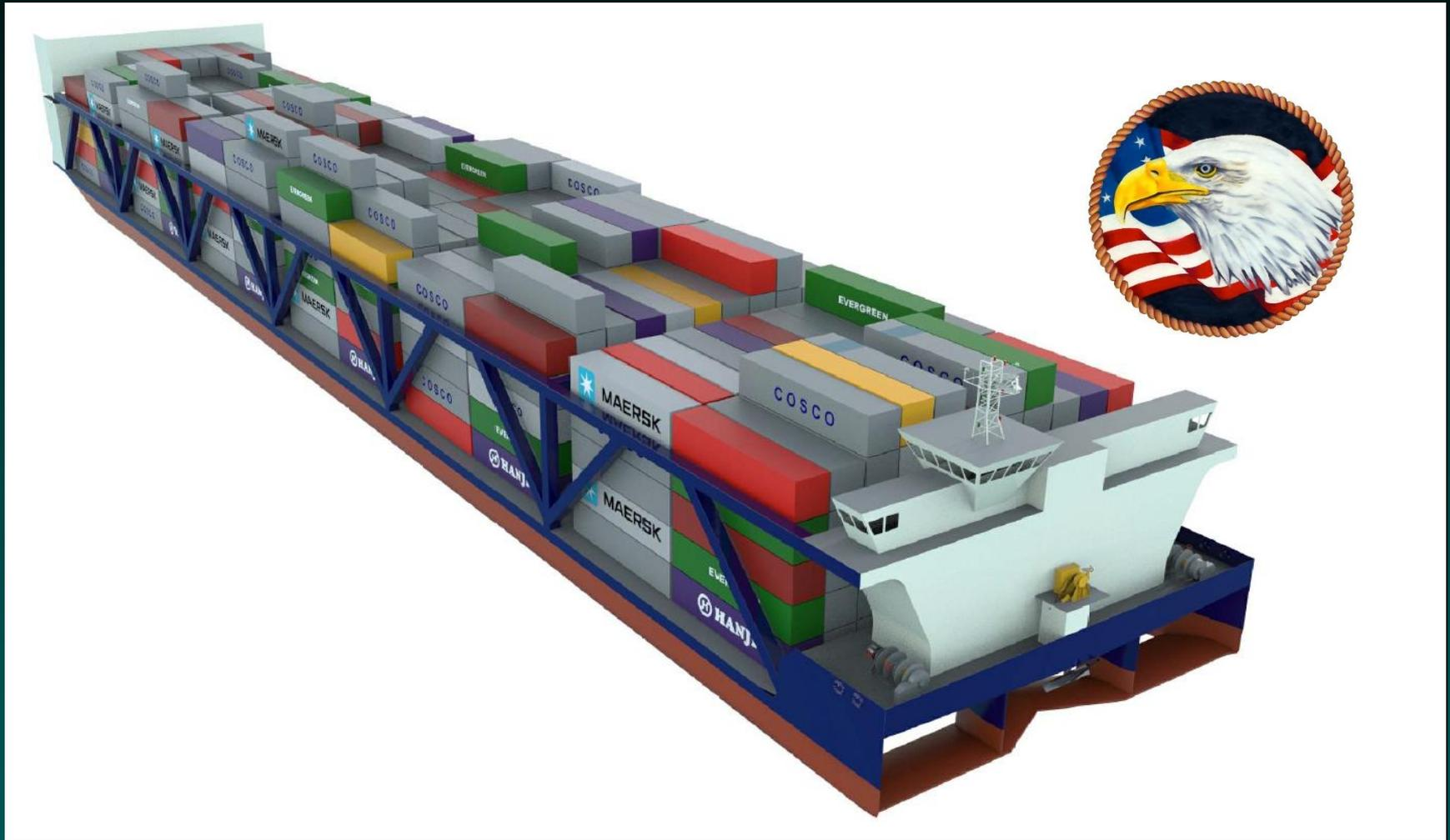
A “*State of the Art*” Hull Design to Ensure Optimal Speed in All River Conditions Utilizing LNG as Main Propulsion Fuel
