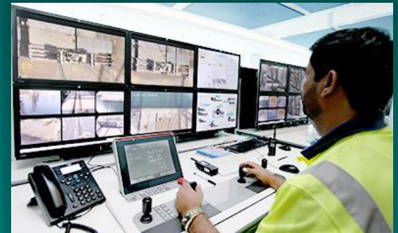
STS Crane Operations from Remote Control Room
