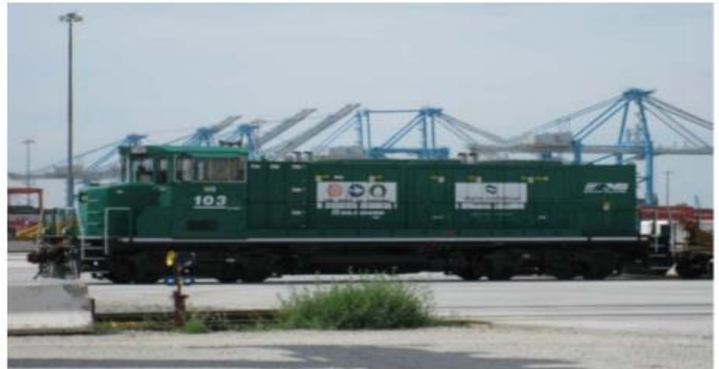
One of two multi gen-set locomotives at NIT
