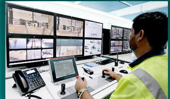
STS Crane Operations from Remote Control Room
