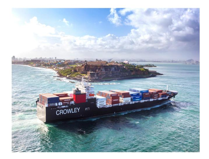
One of the world's first combo roll on/roll off ships powered by LNG.
