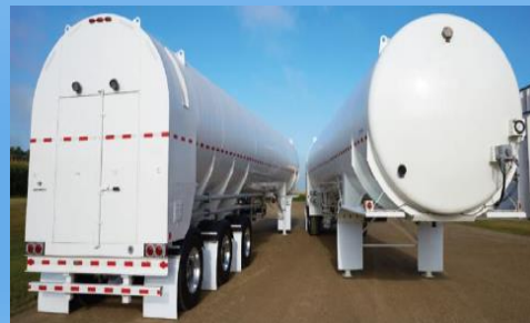
MC-338 Truck Cargo Tank Capacity: ~11k gallons
