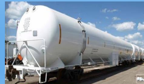
DOT 113 Rail Tank Car Capacity: 15k-30k gallons
