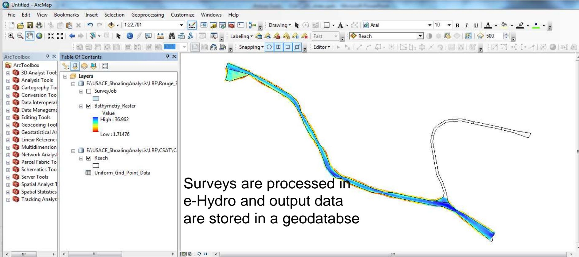
Surveys are processed in e-Hydro and output data are stored in a geodatabase
