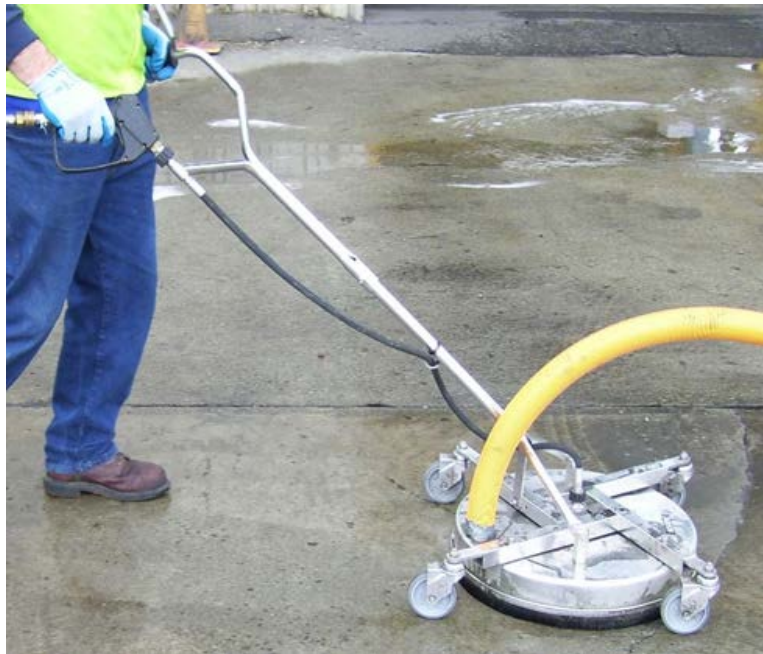
Figure 1 - Dock Scrubber Unit
