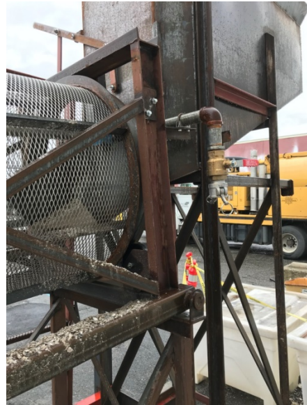
Figure B-2 - Water Inlet Connection
