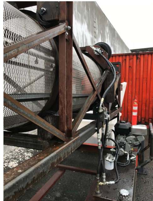
Figure B-4 - Motor Attachment
