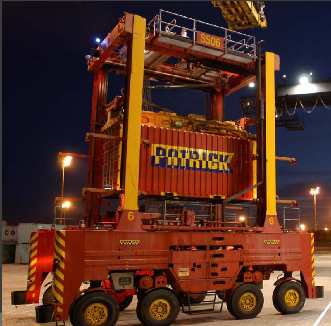
Driverless Straddle Carrier at Patrick Terminal, Australia
