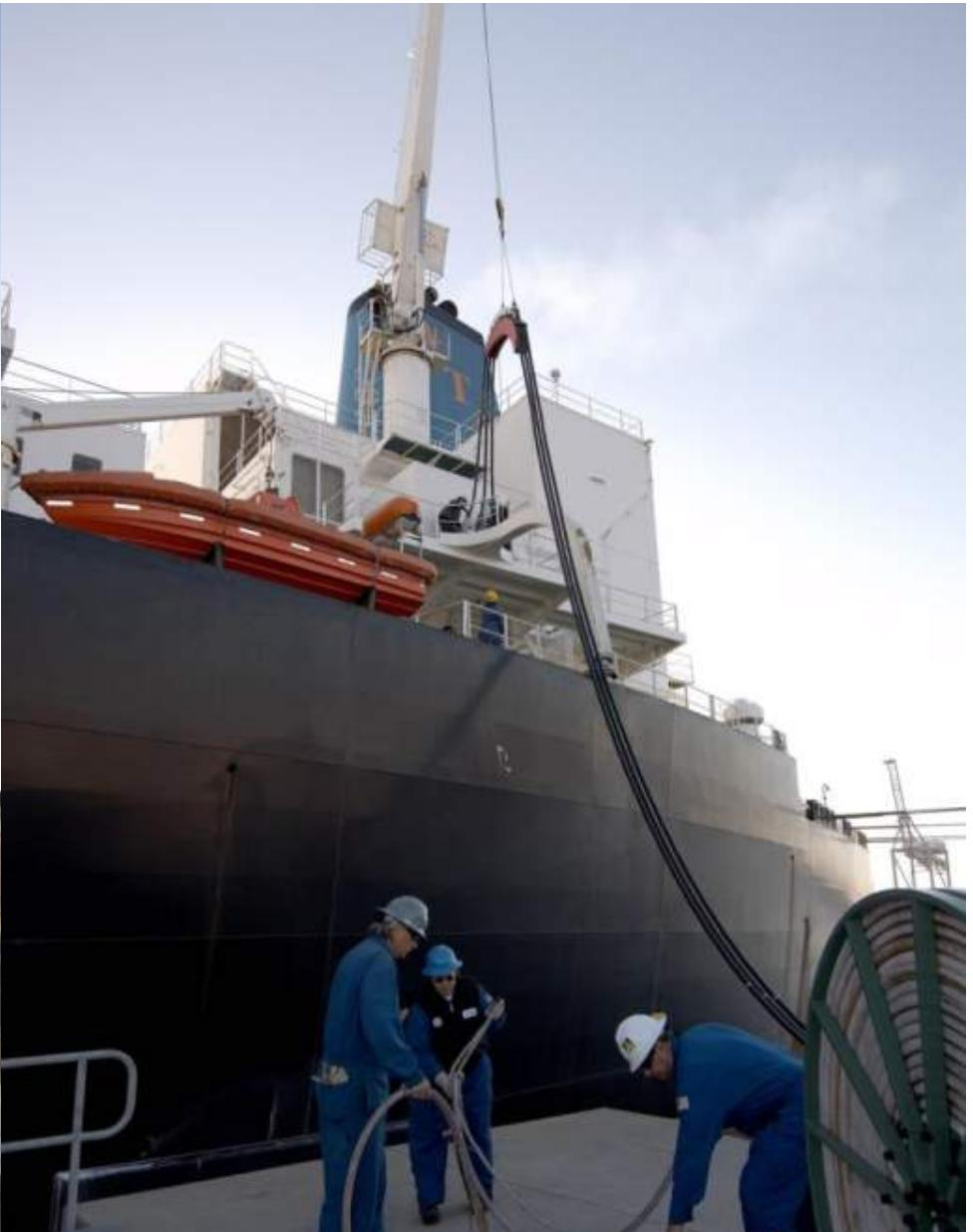
Shore electricity for “K” Line container ships beginning October 2008; for BP oil tankers beginning June 2009
