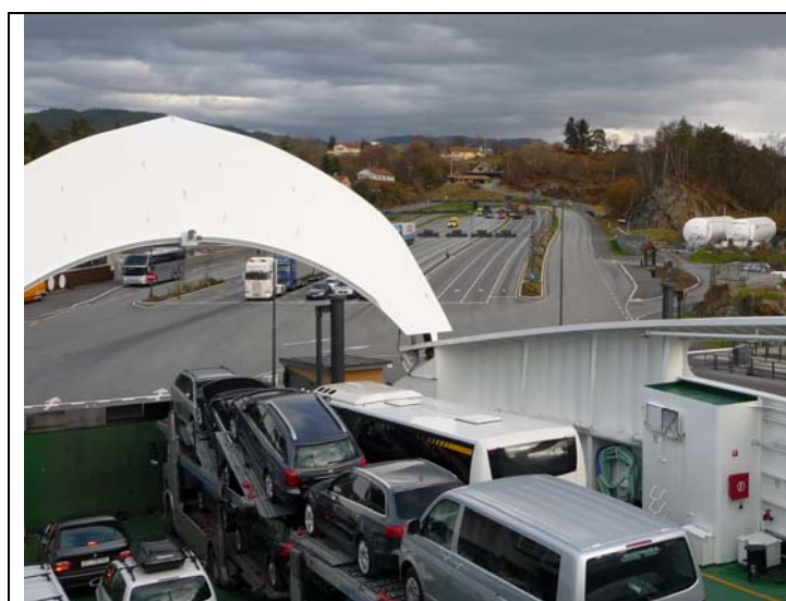
Figure 7-1 The gas fuel led ferries Bergensfjord, Fanafjord and Raunafjord operating between Halhjem and Sandvikvåg have two LNG tanks onboard of 125 m 3 each. For bunkering, two LNG tanks of 500 m 3 each are located on the quay at Halhjem (right). These tanks are refilled by a LNG carrier or trucks (Photo courtesy of DNV)
