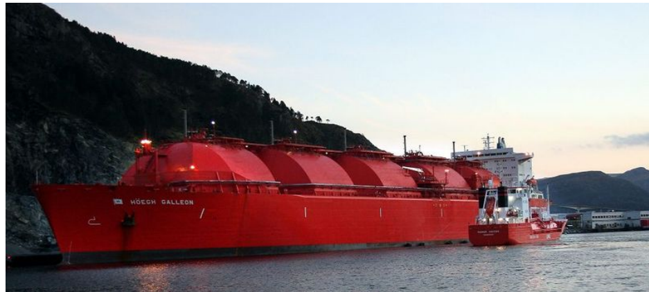
Figure 2-3 Pioneer Knutsen and Höegh Galleon conducting a ship to ship transfer of LNG cargo
