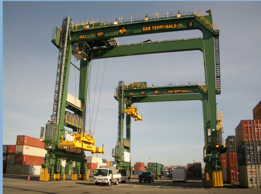
ZPMC Capacitor RTG Seattle, Washington 10% - 13% fuel reduction Significant emissions reduction ~ 20% or more
