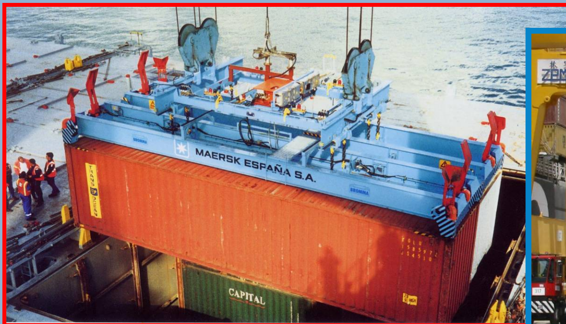
Single Hoist and Head Block Bromma Spreader
