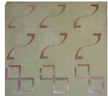
Antennas fabricated on 12"x12" in LCP Film
