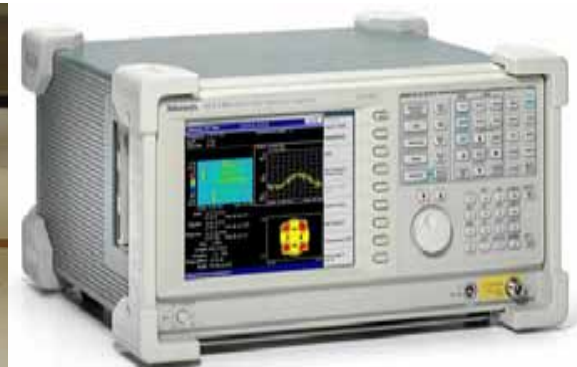
power/freq/time RTSA measurements
