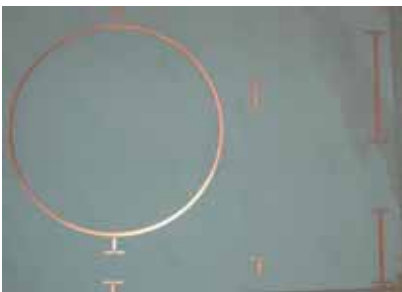
Ring Resonator Method
