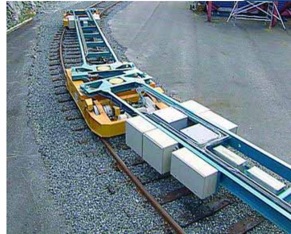
TTS Container Platform-train (CP-train)
