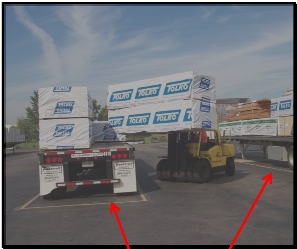
Painted parking locations to ensure adequate space for loading
