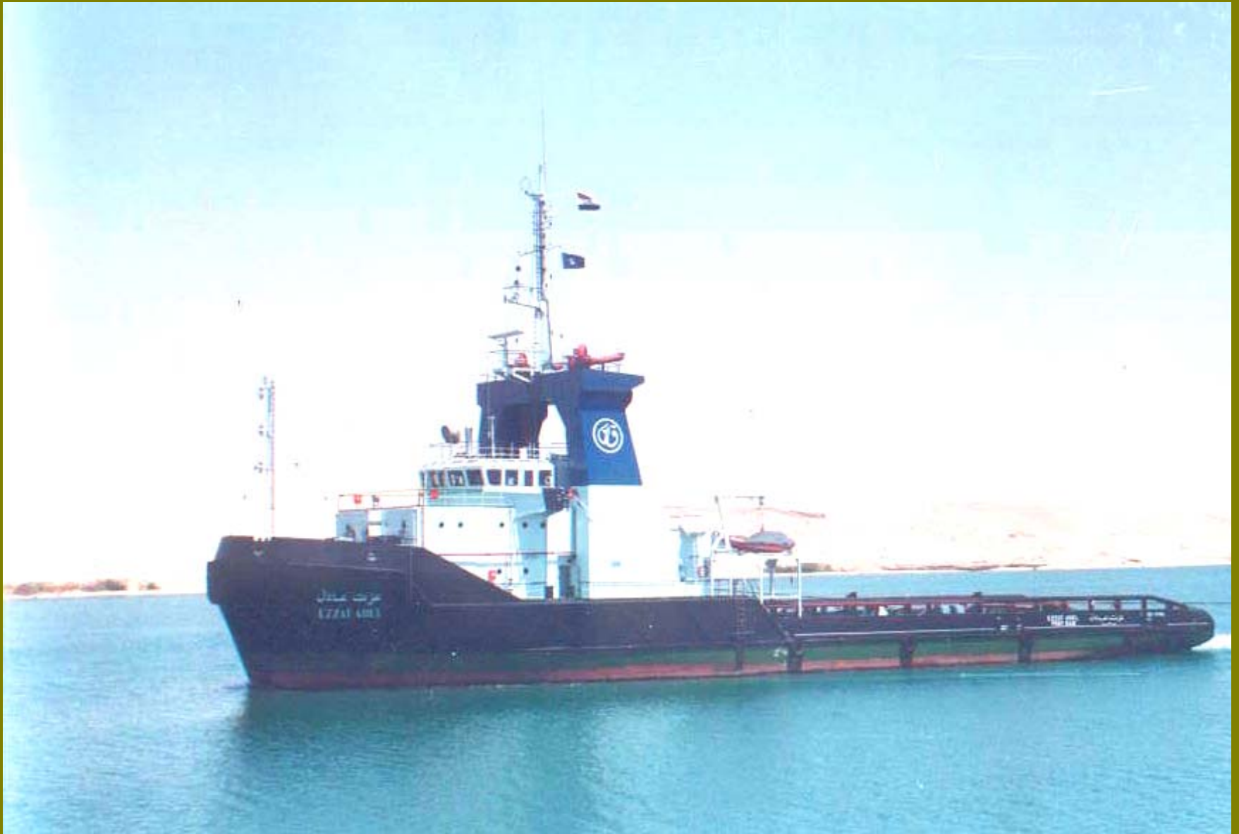
One of the biggest tugs of 160 bollard pull tons
