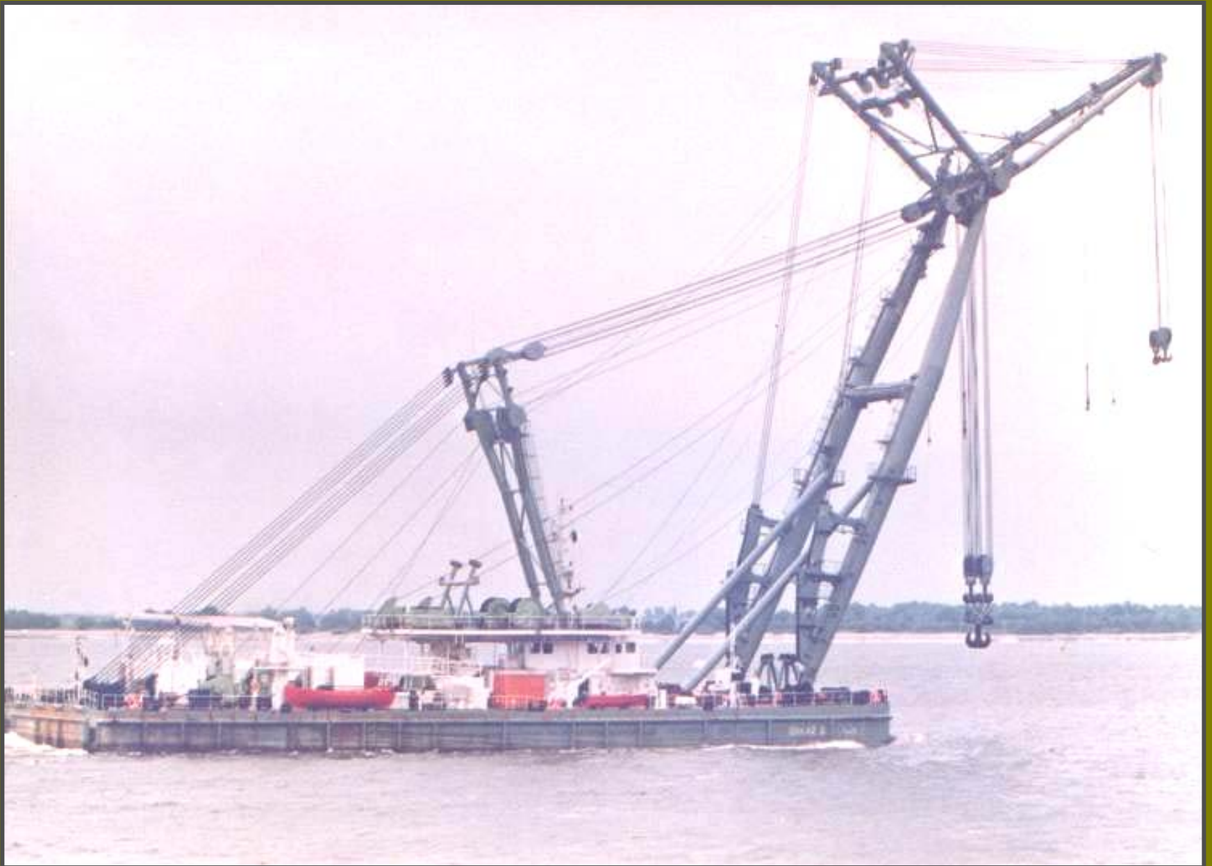
Floating Crane Enkaz 500 tons
