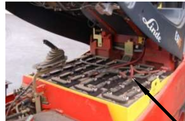
Fork Lift Batteries
