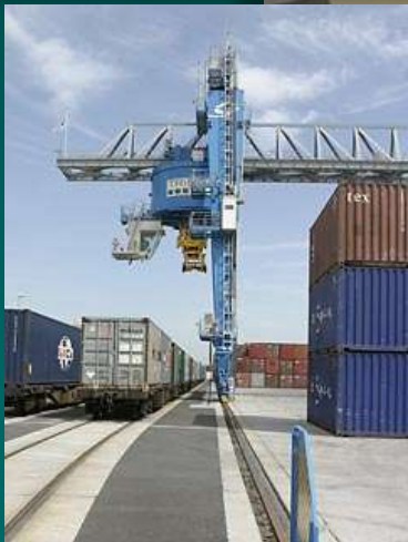
Automatic Stacking Cranes (ASC)
