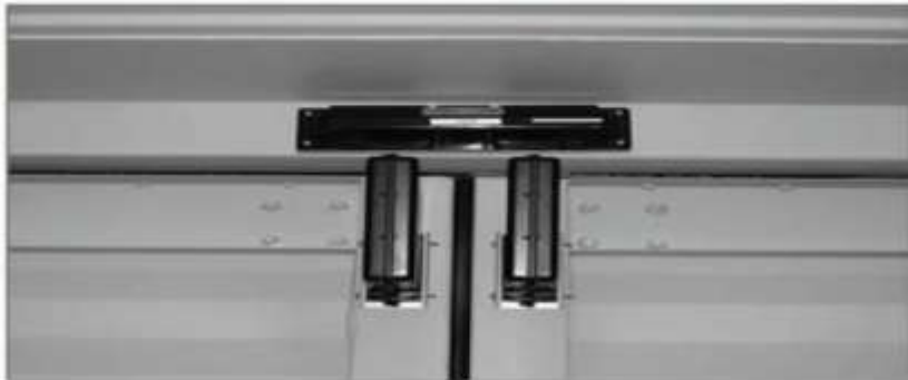
GTRI CSD mounted inside a container.
