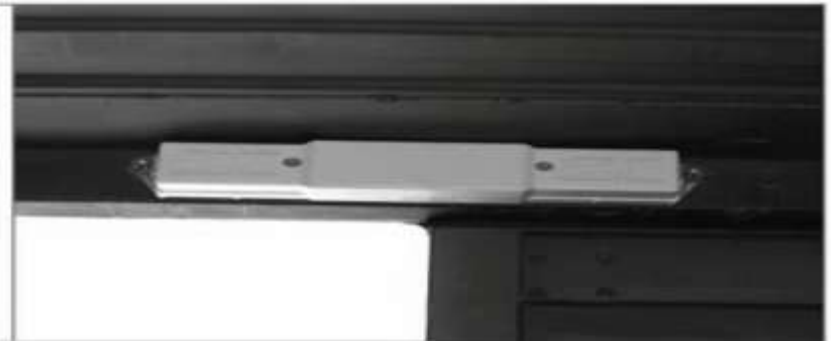
SAIC CSD mounted inside a container, above container doors.
