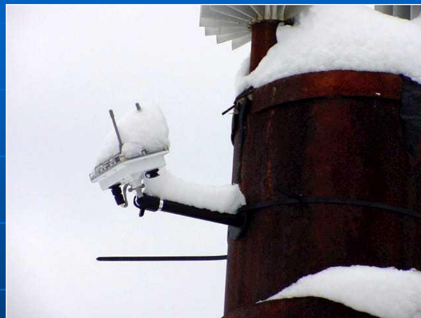
Sensor Web Pod attached to Alaska Pipeline (Fairbanks, AK)
