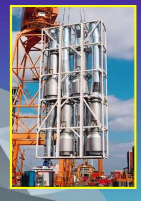
Scrubber also removes most of the particulates PM is removed from the discharge and disposed at dock
