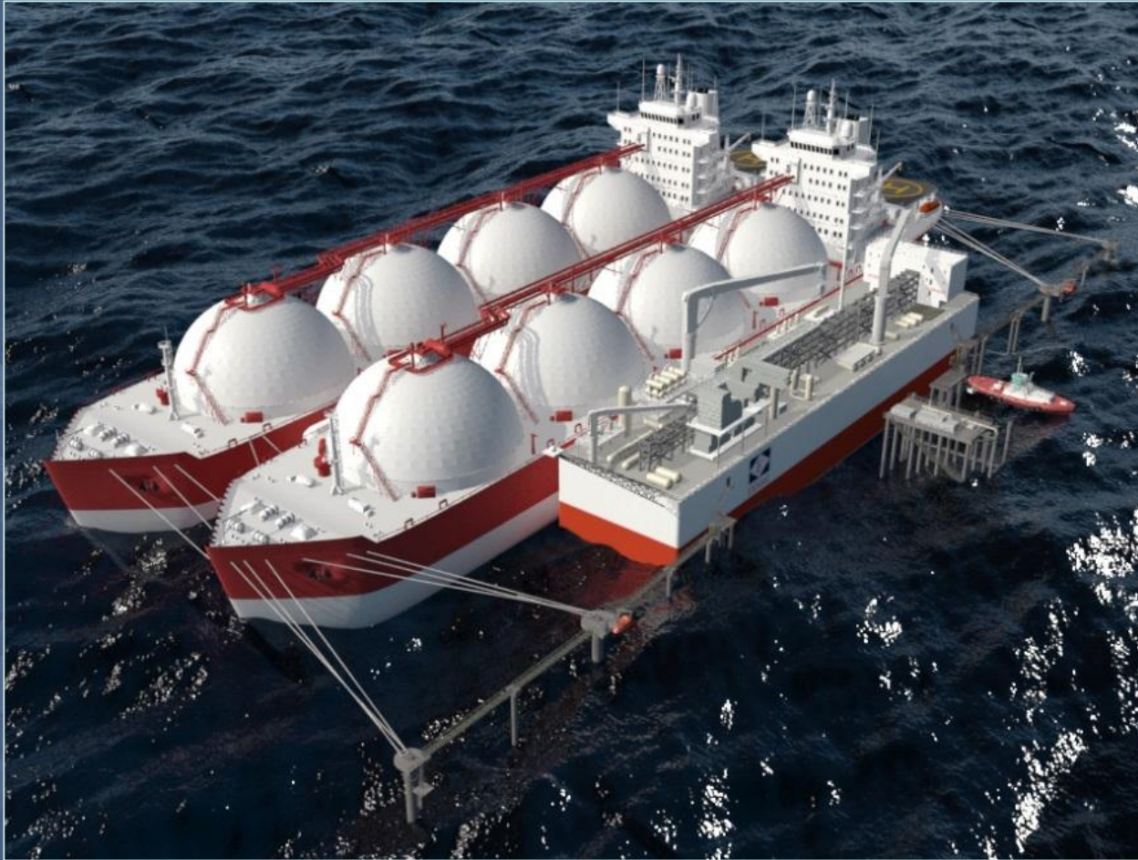
Floating Liquefaction Barge with FSU and LNG Carrier
