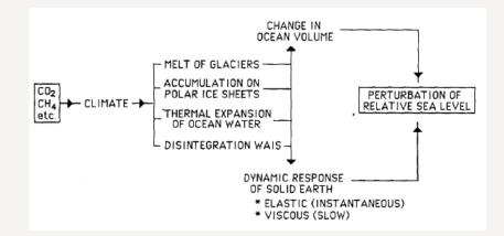
Most important process that determine a change in relative sea-level. After Oerlemans (1989)
