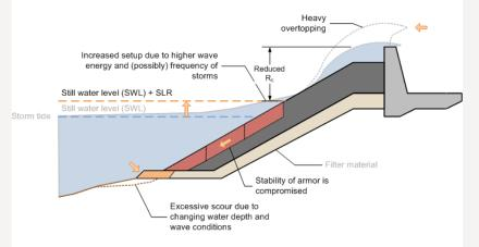
Response of engineered structures to changes in sea-level
