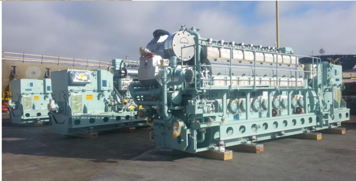
Dual Fuel Diesel Generators (DFDG)
