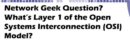
**Physical:** Transmission and reception of raw bit streams over a physical medium.
