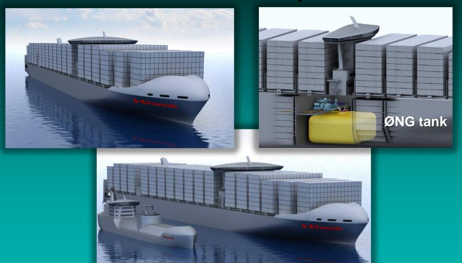
A new type of LNG tank that provides more space for container cargo.
