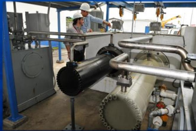
Prototype testing of hydraulic cylinders for gates
