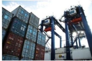
4 Electric Rubber-tyred Gantry Cranes
