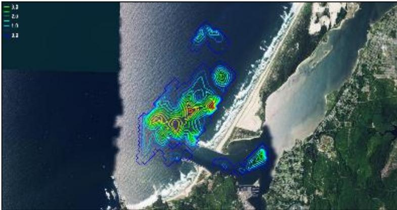
Sediment containing tracers is placed in both nearshore and offshore ODMDS and tracked over time
