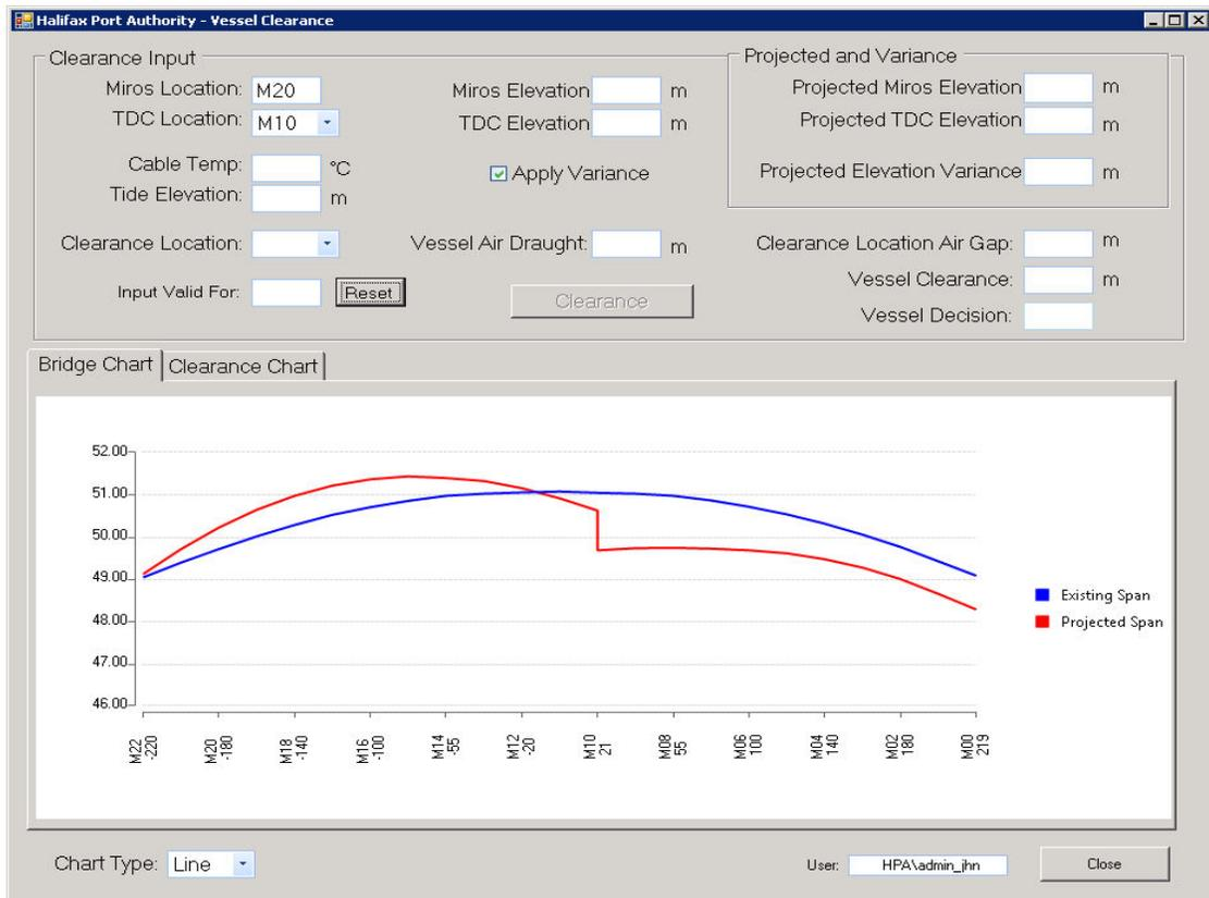
**Figure 7 – Vessel Clearance System Screen**
