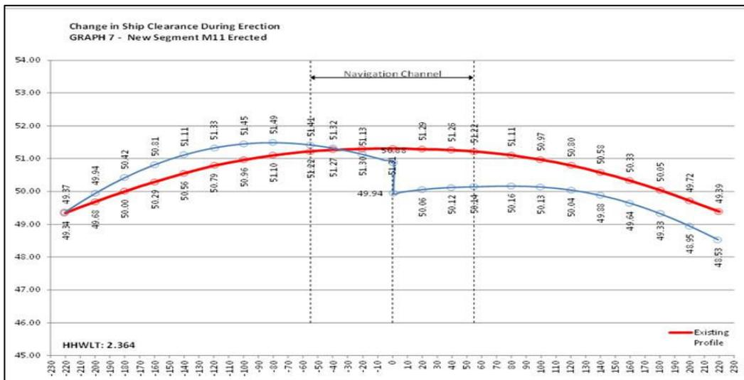
**Figure 2 – Change in Bridge Geometry at Mid-Span**
