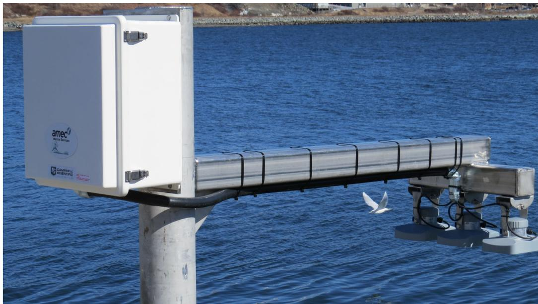
**Figure 4 – OTT RLS Radar Water Level Sensors**
