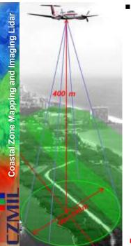
3<sup>rd</sup> generation coastal mapping and tactical charting system Collects bathymetry up to 60 m Engineering scale survey accuracy
