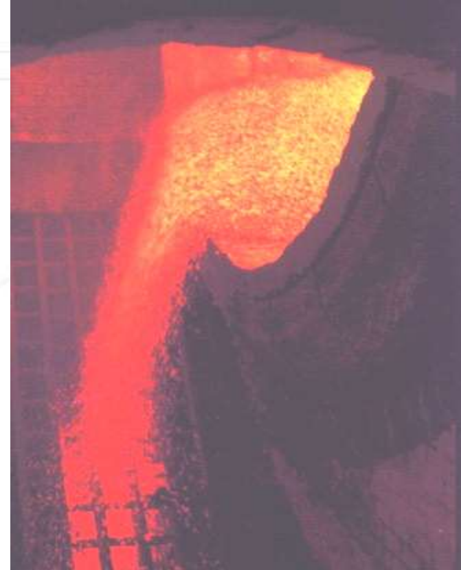
LWA exiting rotary kiln
