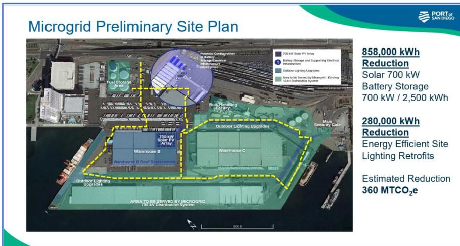
providing back-up power to security infrastructure, site lighting, and the existing jet fuel storage system, which services the San Diego International Airport. In addition, this includes a
