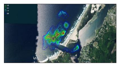
Sediment containing tracers is placed in both nearshore and offshore ODMDS and tracked over time
