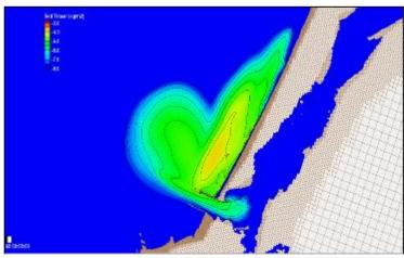
Coastal Modeling System predicts sediment movement and results are verified with field observations
